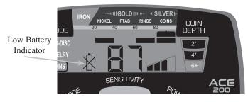
The Low Battery Indicator will switch on when the detector's batteries become weak. The detector will maintain full performance but the batteries should be replaced soon when this indicator appears. NiMH rechargeable batteries may be used, but may have a shorter life per charge. You can expect 20 to 40 hours of operation depending on battery type and quality.
